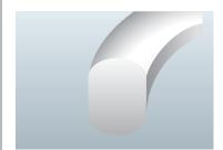
This gasket is made of forged metal formed into an oval cross-section.
